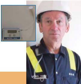
As shown in Photos 1 and 2, the datalogging instrument was taped into the upper pocket of coveralls and the remote sampling probe was positioned on the top of the shoulder. In this location, the device is protected and the alarm is easily heard.
