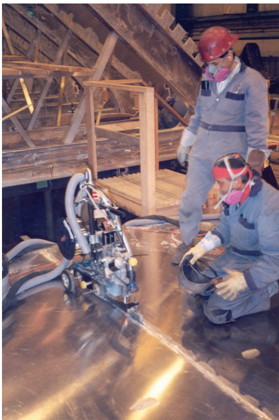
Fig. 1 — A2 welding machine prior to installation of fume collector hood.
