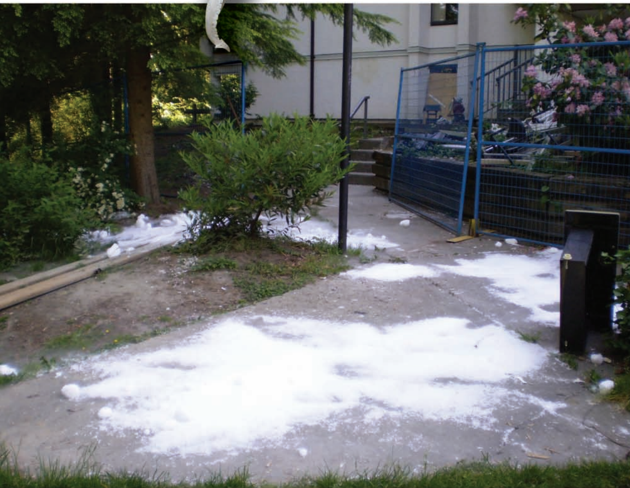
Figure 1: Dry ice is not ice! Waste dry ice spread on the ground, as shown here, can generate a cloud of carbon dioxide having high concentrations. In this example, the concentration of CO 2 was 2500 ppm at chest height in the early morning in late spring.
