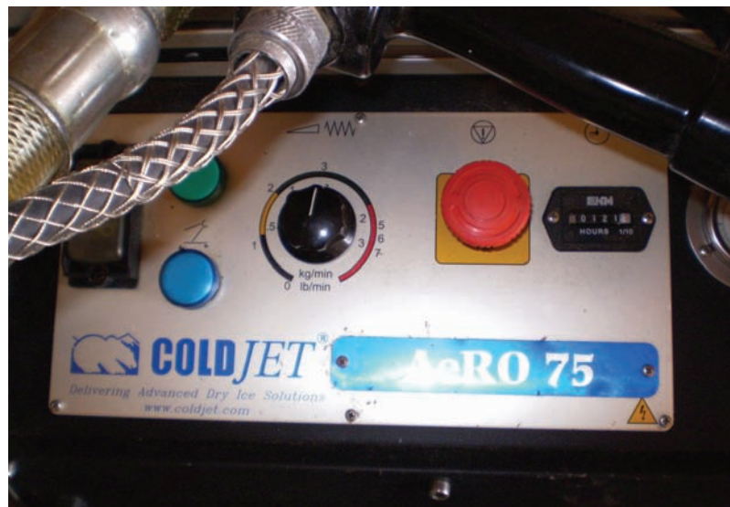
Figure 3: Dry ice delivery. A delivery rate of 3 lb/min (1.4 kg/min) of dry ice corresponds to production of 25 ft 3 /min of CO 2 gas by sublimation. This requires a minimum ventilation rate of 5040 ft 3 /min under ideal conditions to dilute the concentration to 5000 ppm. Displacement ventilation may require less air flow.
