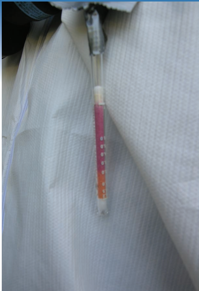
Figure 5: Monitoring exposure to CO 2 using passive dosimeter tubes. Passive dosimeter tubes provide an inexpensive way to monitor exposure to CO 2 during abrasive blasting using dry ice. The change in color indicates exposure in % • hours (1 % = 10000 ppm) on the scale printed on the tube. This method can provide considerable information when regular periodic observation of the tube and recordkeeping occur during the work.
